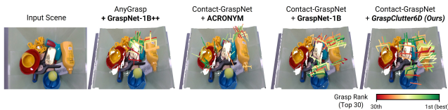
Fig. 9: Grasp predictions (top 30) in a real-world pile scene .
